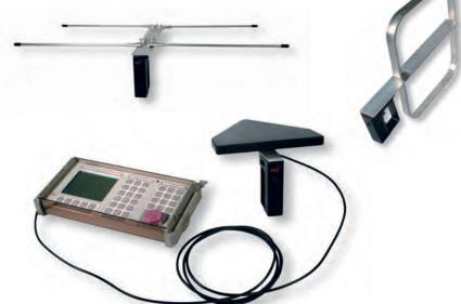
for 20 Mhz up to 250 MHz Directional antenna 3: for 200 MHz up to 500 MHz Directional antenna 4: for 400 MHz up to 6 GHz These have to be connected to analyser. A complete scan needs less than 500 ms at high resolution. Even sources with very low transmitting power can be identified using the directional antennas due to their extreme low noise level of -30 dB $\mu$ V/m.
