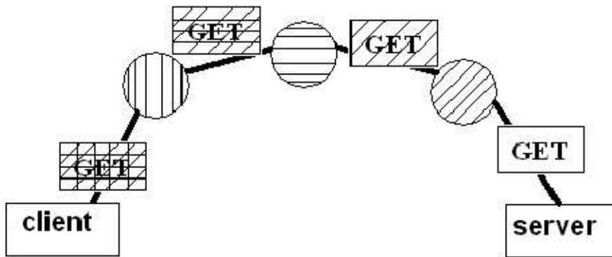
Figure 2: (U//FOUO) Layers of encryption on a normal GET.
